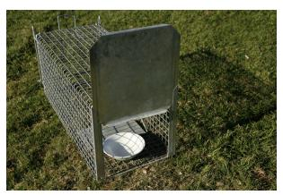
4. Push down on handle and prepare to set trigger on trap. Trap should look like this once set. Hook trigger over handle. Tray at bottom of cage should be raised slightly.
